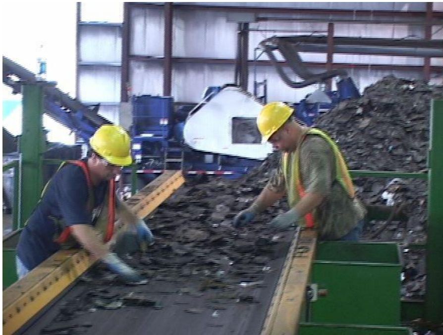
Figure 2. Post-consumer shingle manual sorting
