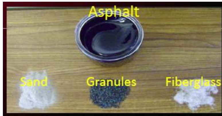
Figure 1. Components of Asphalt Shingles (Grzybowski et al. 2010)
